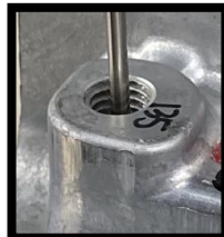
Inverter Housing (M6 Threaded Hole) — Porosity Inspection Image
